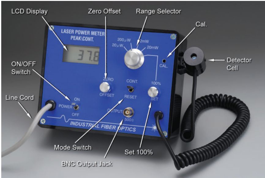
Figure 2. Front view of digital power meter.
